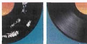
(Left) Styrofoam beads are attracted to static charge left on record after cleaning with Discwasher D3®.
